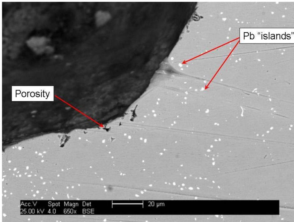
*Structure of brass revealed in scanning electron imaging, using back-scattered electrons. Polished section cut through a leaded brass faucet.*
