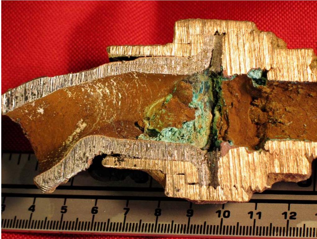
*Build up of excess scale at the junction between Pb pipe and brass fitting. The brown scale to the left is dominantly PbO<sub>2</sub> with some white Pb carbonate underneath, whereas the scale to the right, on the brass, is dominantly Mn oxide. At the junction, Cu sulfate dominates.*
