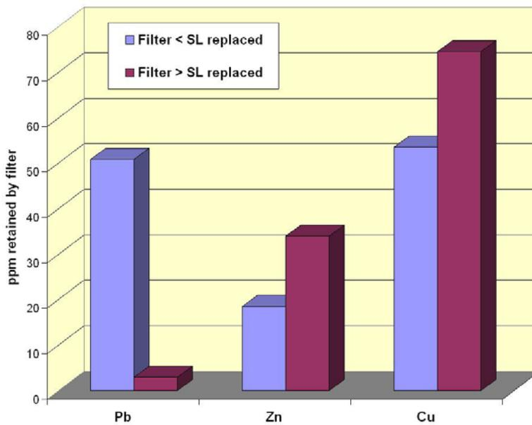
*Removing the service line (SL) dramatically reduces the amount of lead (Pb) entering the house*
