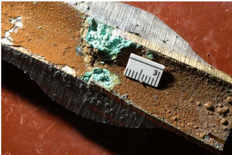
system are various brass components – the curb stop valve, the meter, and the shutoff valve in the house. Thus a Pb supply line will have a number of brass connections along its length. These bimetallic connections have the potential for accelerated galvanic corrosion, as illustrated below.
