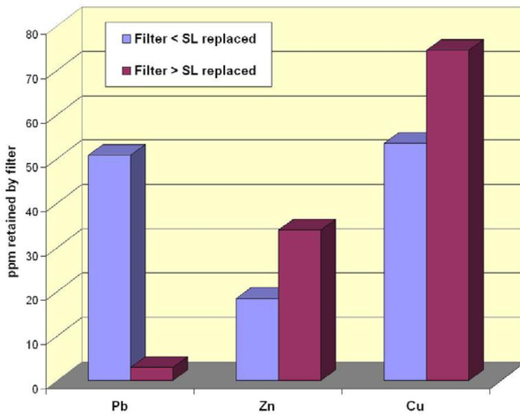
*Removing the service line (SL) dramatically reduces the amount of lead (Pb) entering the house*
