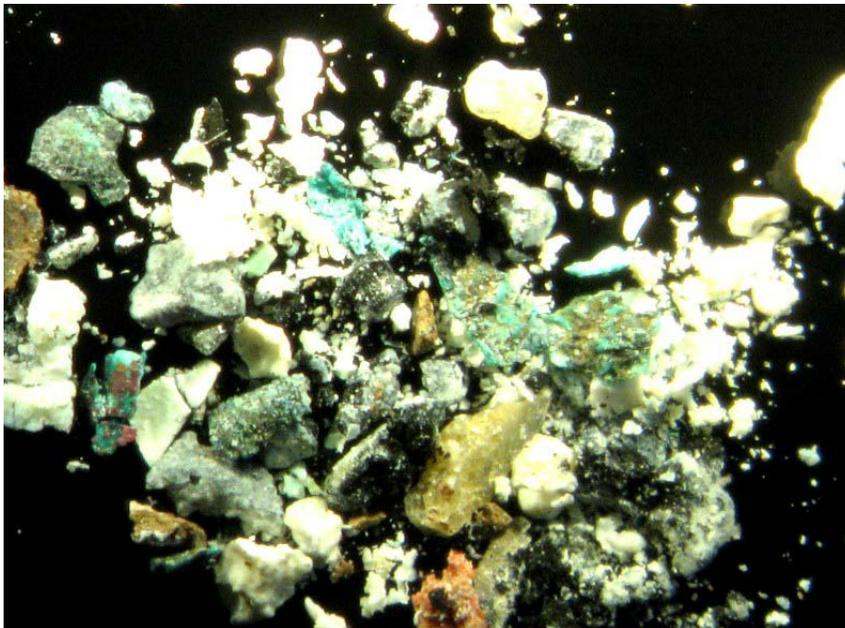
*Debris recovered from a kitchen faucet aerator. The green particles are copper rich, the white particles are zinc-rich and the reddish particles are iron oxide with some lead.*
